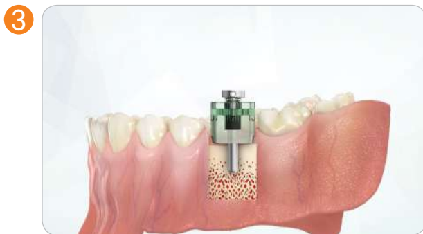
3 Insert the Guide Pole(or Guide Pin) to the all of drilling hole to path check (if necessary, taking an X-ray)
